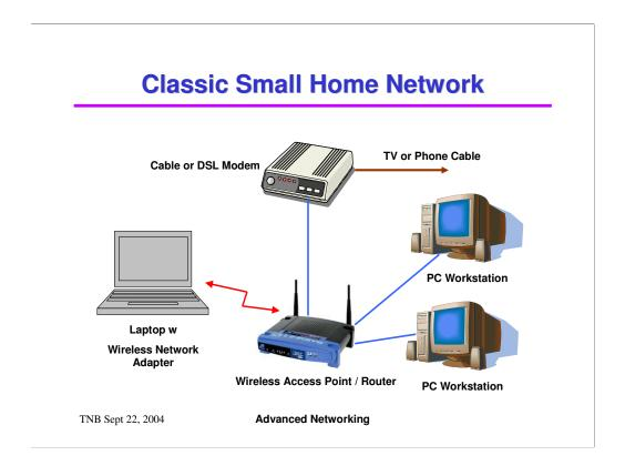
Above is the archetypical simple mixed wired and wireless network configuration diagram.
