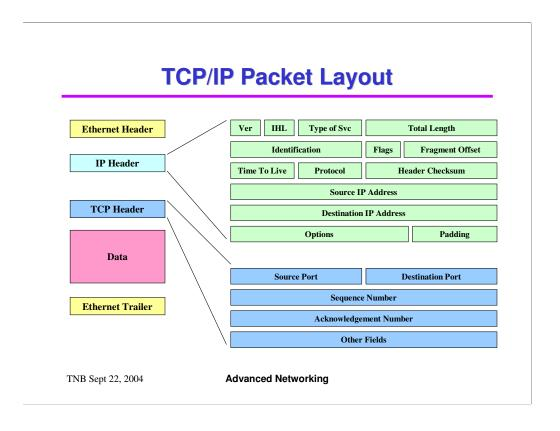
The above diagram shows the block layout of a packet.
