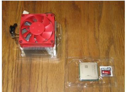
Here are the AMD A10-7860 CPU and its heat-sink cooler. These will be mounted on the motherboard.
