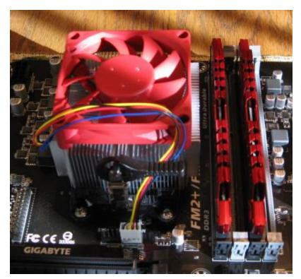
There are springy flat metal clamps on each side of the heat sink with holes that fit over two ears on the base of the socket. Settle the heat sink in place, engage the hole in one the clamps over a socket ear. Then press down gently and engage the second clamp's hole over the other socket ear. Finally, swing the black cam lever to the position shown, which will tighten the clamps and force the heat-sink tightly against the CPU.
