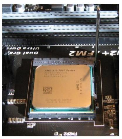
Once the CPU chip is in place, lower the lever arm and latch it. This will clamp the chip in place and ensure all pins have made good contact.
