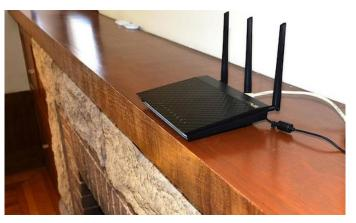
Radio waves travel best through open air, so sight lines are a good clue here: if you can see the router from far away, and from many different angles, you're using it efficiently.
